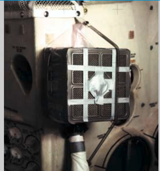
The astronauts used cardboard, plastic bags, and tape to create a device to make the air breathable.
